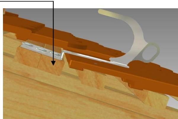
2. Fix the LUX - top® SDH-B as shown in the following installation sketch using the three woodscrews **8.0 x L** mm supplied without predrilling; fix on the lathing in the middle of the rafters (min. 6/14 cm; min. strength class C 24 to DIN EN 338).
